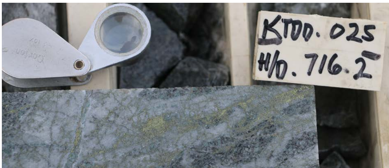
Chalcopyrite rich mineralisation in drill core KTDD025.
