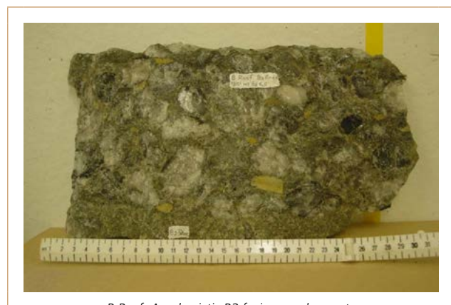
B Reef: A polymictic B3 facies conglomerate with khaki coloured shale clasts matrix.
