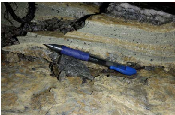
Ultracataclasite fault rock above Vaal Reef.
