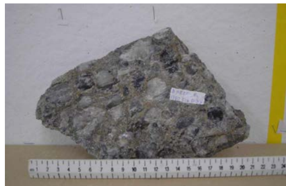
B Reef: A hand sample of B1 facies conglomerate form 1750 E14 Drive S3.
