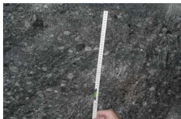
B Reef: An oligomictic, matrix-supported B1 facies conglomerate.
