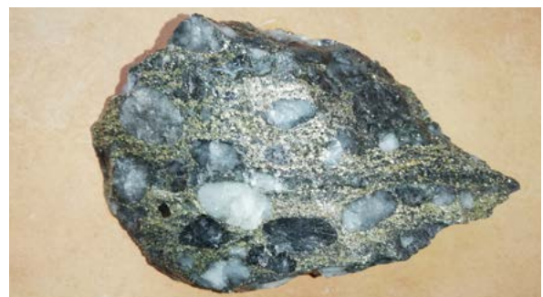
Beatrix Reef with argillaceous matrix and pyrite stringers.
