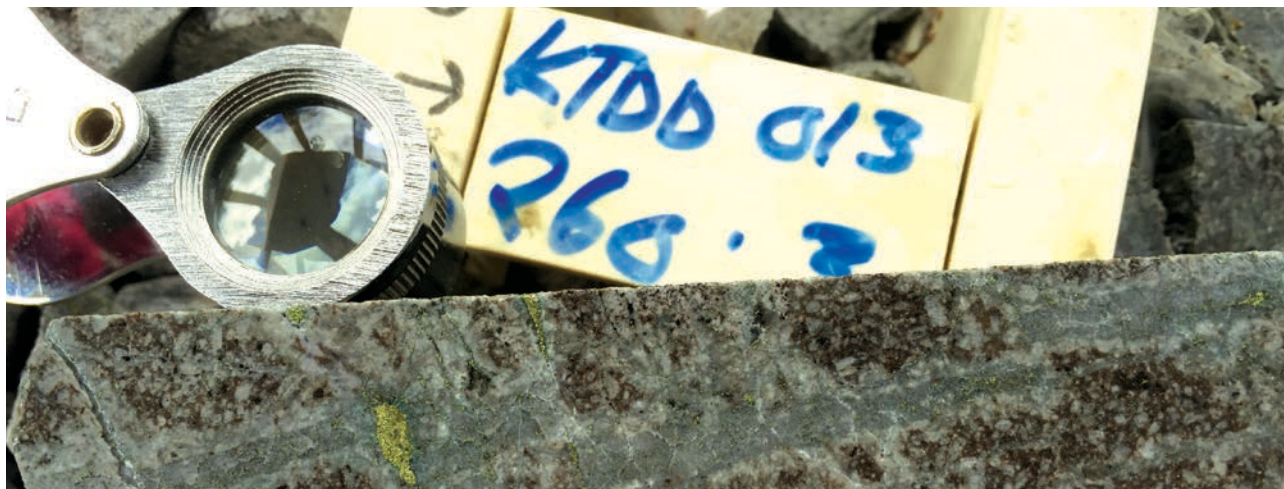
Drill core from KTDD013: 260.3m, Quartz vein stockwork with chalcopyrite developed in pervasive biotite (potassic) altered diorite porphyry
