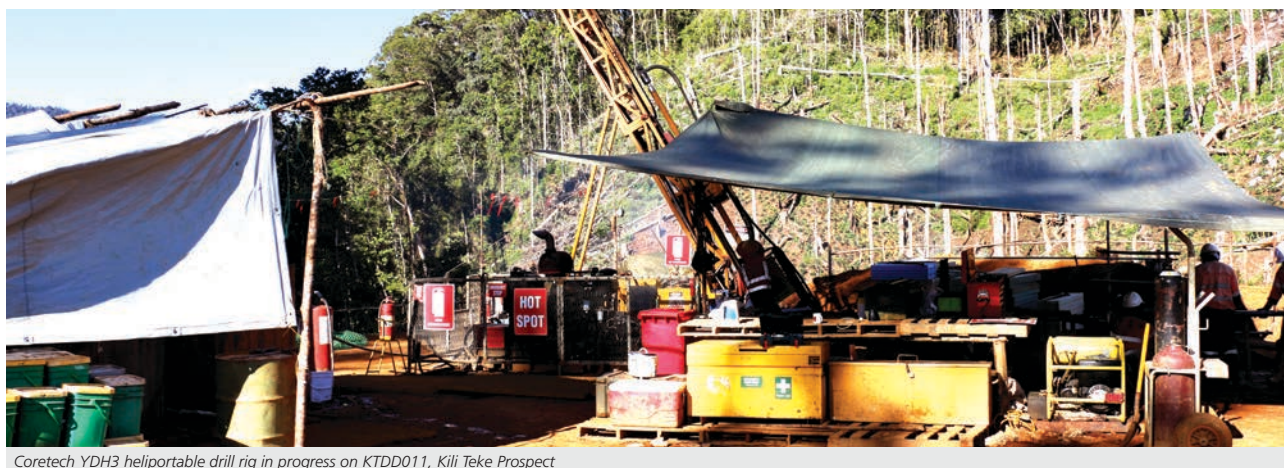
Coretech YDH3 heliportable drill rig in progress on KTDD011, Kili Teke Prospect
